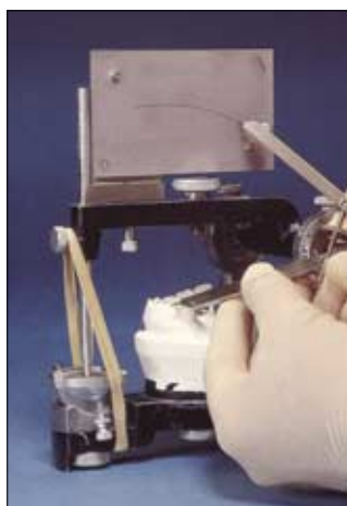
Fig. 3 An arc is drawn on the flag at a set radius using the tip of the lower canine as its centre (Canine Arc)
