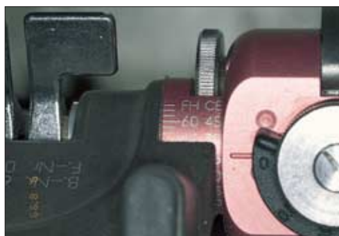
Fig. 16b ...indicating that the condylar angle is 45° (scale FH) Frankfurt Horizontal (KaVo Articulator)
